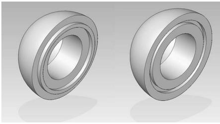
FIG. 3. Modified design of neutrally buoyant spheres, showing the two halves which connect together.
